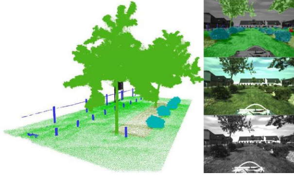
Figure 6. Overview of the 3DRMS Challenge dataset: training sequence "boxhood row" with the 3D semantized point cloud and on right column 2D semantic annotations over image, front-left RGB image, front-right grayscale image.
