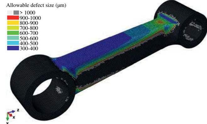
Fig. 19. Allowable defect size distribution on the crank model.
