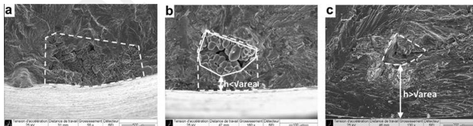
Fig. 11. Measurement of defect size. (a) surface defect; (b) defect close to the free surface; (c) defect far from the free surface.
