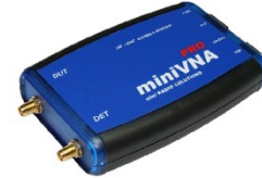
Figure 5. Photograph of the network analyzers used in the experiment: the mini-VNA PRO.
