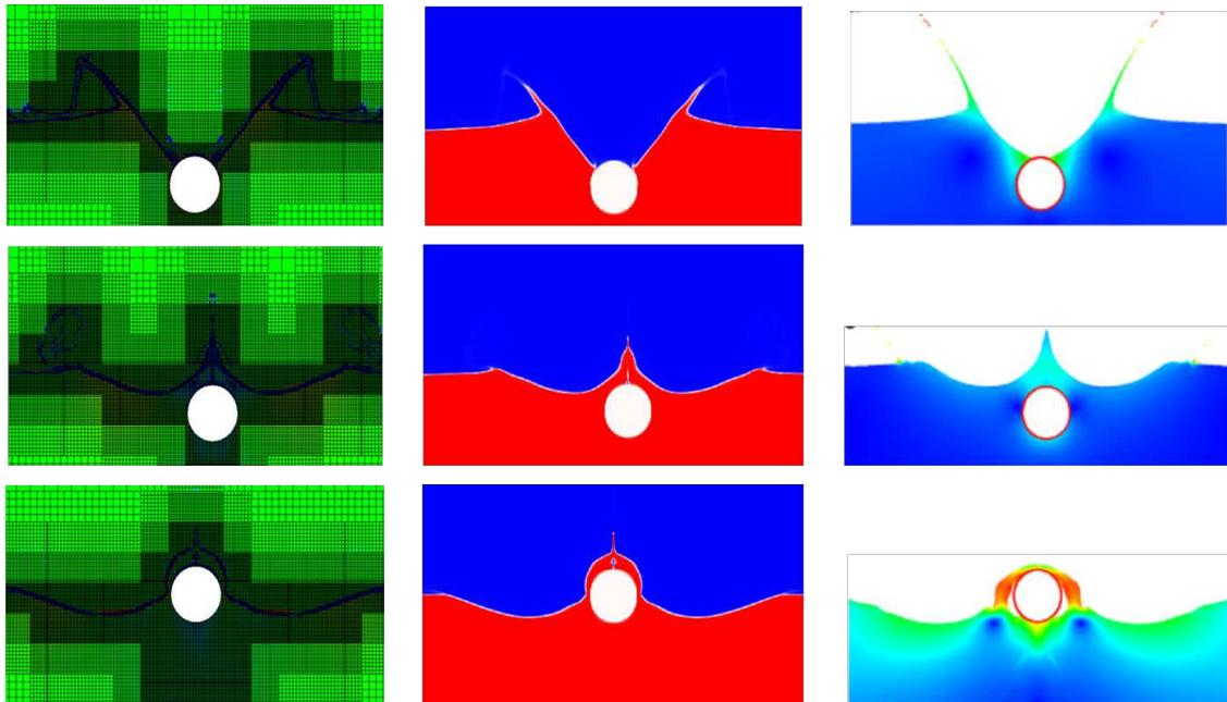
Figure 5: Water entry of half buoyant cylinder at  $t = 0.37s, t = 0.63s, t = 0.77s$ . Left: mesh and numerical production of entropy (green: zero, blue: negative value). Middle: density (red:water, blue:air). Right: results of Sun and al. [23] using SPH method.
