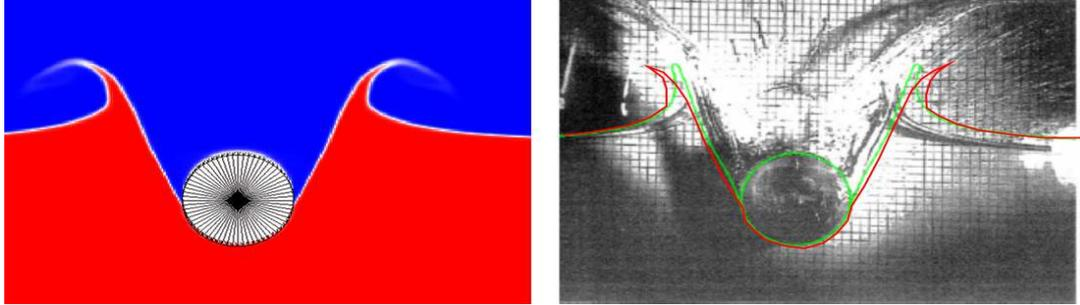
Figure 4: Penetration of the cylinder at  $t = 0.385s$ . Left: present numerical simulation. Right: Experiment [12], free surface profile of present numerical simulation with red solid line, free surface profile of BEM results by [22] with green solid line.
