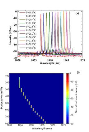
Fig. 3. Optical spectrum tunability of the VECSEL by setting different operation temperature at 600 mW of pump power (a) and the recorded emitting wavelength at various pump powers (b).
