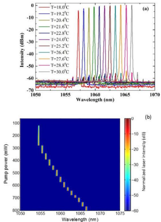
Fig. 3. Optical spectrum tunability of the VECSEL by setting different operation temperature at 600 mW of pump power (a) and the recorded emitting wavelength at various pump powers (b).
