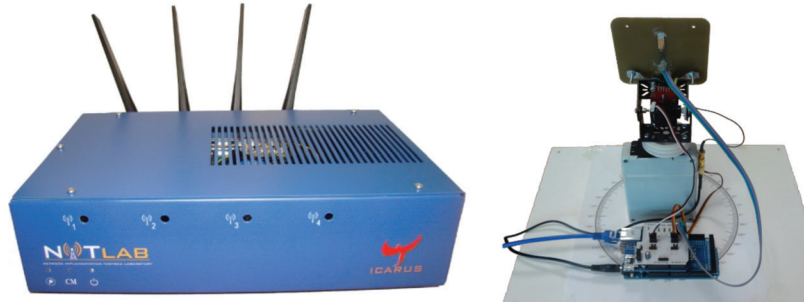
Figure 12.5 Extensions of the NITOS testbed: Icarus nodes on the left and directional antennas on the right.
