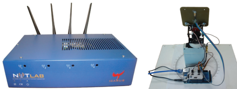
Figure 12.5 Extensions of the NITOS testbed: Icarus nodes on the left and directional antennas on the right.
