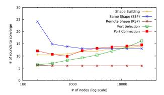
Figure 10: Convergence time of the PLEIADES protocols for a system of 20 connected rings (a *ring of rings*), for various system sizes. PLEIADES converges rapidly and scales well with the number of nodes.
