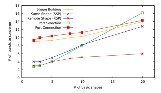
Figure 11: Convergence time of the PLEIADES protocols for a system of 25,600 nodes implementing a *ring of rings*, for various numbers of rings. The convergence time of PLEIADES only slowly increases with the number of individual rings.
