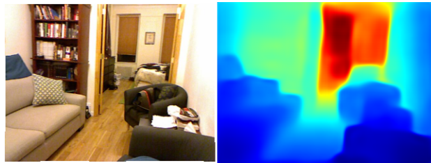
Fig. 1. An example of our state-of-the-art monocular depth estimation trained with a deep multi-scale architecture.
