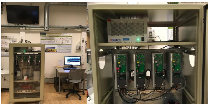
Fig. 1. Microgrid emulation module for experimental tests ( Microgrids group, Aalborg University )
