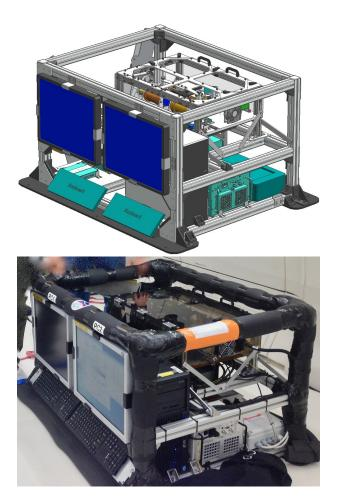
FIG. 4. Top: Drawing of the instrument rack by DTM Technologies<sup>TM</sup>. Bottom: Picture of the rack onboard the aircraft.
