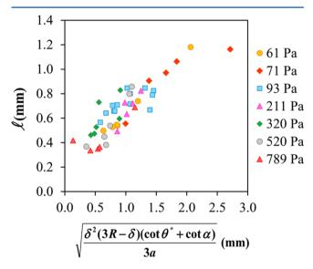
**Figure 7.** Experimentally measured foot length l as a function of a combination of the relevant geometrical parameters, according to eq 7. The shear moduli are indicated in the legend.
