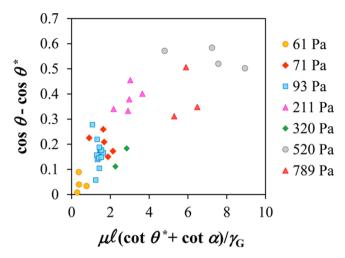
**Figure 4.** Experimentally measured difference between the cosines of the contact angle  $(\theta)$  of water and the contact angle  $(\theta^*)$  of hydrogel, plotted according to eq 4. The shear moduli are indicated in the legend.
