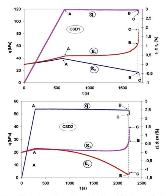
Figure 2. Evolution of the variables q and  $\varepsilon_v$  versus time. The material is stable during AB and the test is controllable. Collapse occurs at point B, the test is no more controllable during BC and the axial strain rate increases.
