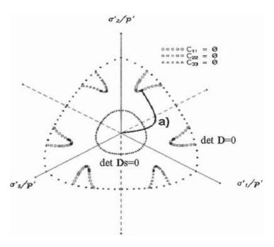
Figure 9. Loci of loss of controllability under different loading programmes (controllability of path is lost when  $C_{11}=0$ ) (from [16]).
