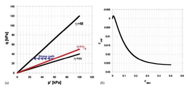
Figure 11. Theoretical predictions in a q constant stress controlled drained test: (a) stress path and (b) volumetric strains.
