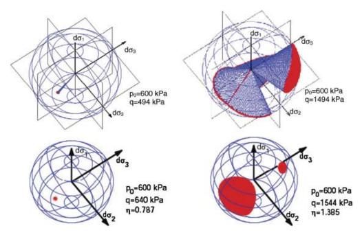
Figure 18. 3D cones of unstable stress directions for a dense sand of Hostun. On the top the cones obtained with the octo-linear model. The planes represent the limit between the eight tensorial zones, the meshes correspond to the analytical solution of Equation (80). On the bottom results obtained with the non-linear model using the numerical method. The point clouds represent the solution plotted on the sphere.  $p_o$  is the initial confining pressure,  $q = \sigma_1 - \sigma_3$ .
