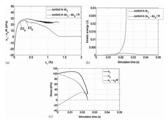
Figure 6. (a), (b) Comparison of simulated responses for a proportion strain loading path controlled by  $\varepsilon_1$  or  $\xi_1 = \sigma_1 - \sigma_3/R$  and for R = 0.825; (c) stress evolutions for a control with  $\xi_1$ .
