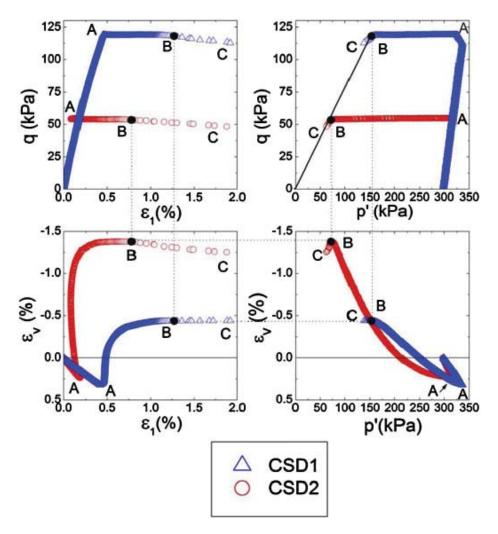
Figure 3. Influence of the control parameters on the mechanical behaviour of Hostun loose sand under q-constant drained tests for two stress ratios  $\eta = 0.17$  and 0.35. Sudden collapse occurs at the minimum of the volumetric strain.
