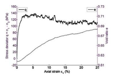
Figure 4. Axisymmetric drained triaxial compression for a confining pressure  $\sigma_3 = 100 \,\mathrm{kPa}$ .
