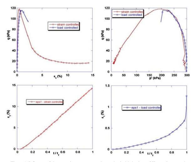
Figure 1. Influence of the control parameters on the mechanical behaviour of Hostun loose sand under undrained triaxial compression tests ( $p'_o = 300 \,\mathrm{kPa}$ ). No sudden collapse is observed for strain-controlled test whereas it occurs at the peak of the load-controlled test when strain rate increases at collapse with decrease in q.
