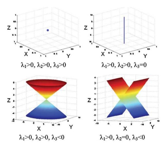
Figure 16. Geometrical representation of the mathematical solutions of Equation (80).  $\lambda_i$  are the eigenvalues of  $\mathbf{C}_s$ .
