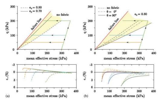
Figure 15. Effect of fabric on the instability response—enlarged bifurcation zone: (a) density level without fabric and (b) consideration of fabric.
