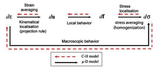
Figure 19. General homogenization/localization scheme relating the incremental stress tensor and the incremental strain tensor.
