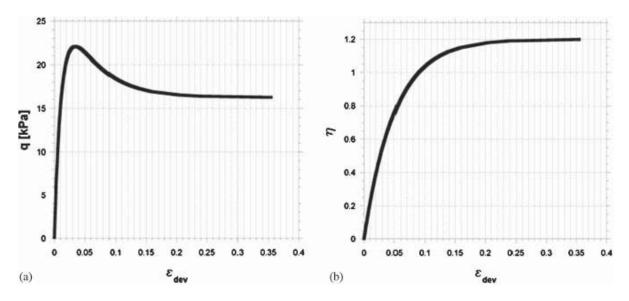
Figure 10. Predictions of an undrained test: (a) deviatoric stress–strain relationship; (b) stress ratio vs strains M = 1.2; m = 0.4;  $\lambda' = 0.09$ ;  $\kappa' = 0.03$ .
