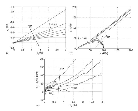
Figure 5. Simulations of proportional strain loading paths for R = 0.7; 0.8; 0.825; 0.85; 0.875; 0.9; 1.0.
