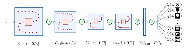
Fig. 3. Architecture of the Q-network. s is the input state (image) and Q(s, x) is the Q-value for action x given state s.  $C_n[f + p/k]$  denotes a convolution layer (using n filters of size f, with a padding of p, and using a stride of k) and  $FC_n$  a fully connected linear layer (of width n).
