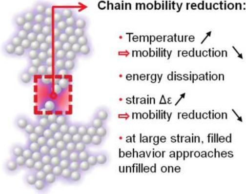
Figure 4. Fillers modify matrix dynamical response: chain mobility reduction: sum up scheme of the chain mobility reduction observations.
