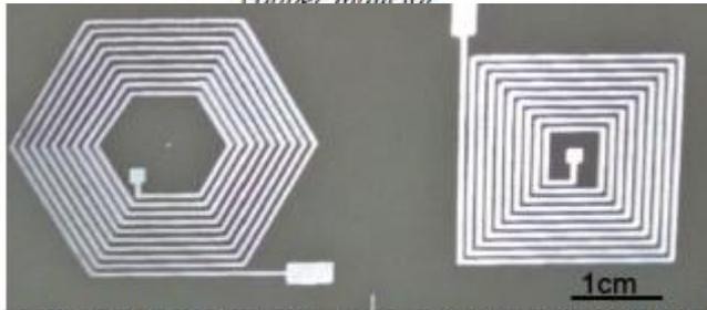
Fig.2 PCB integrated inductors with directly-plated Ni-P magnetic core covered on conductive copper lines
