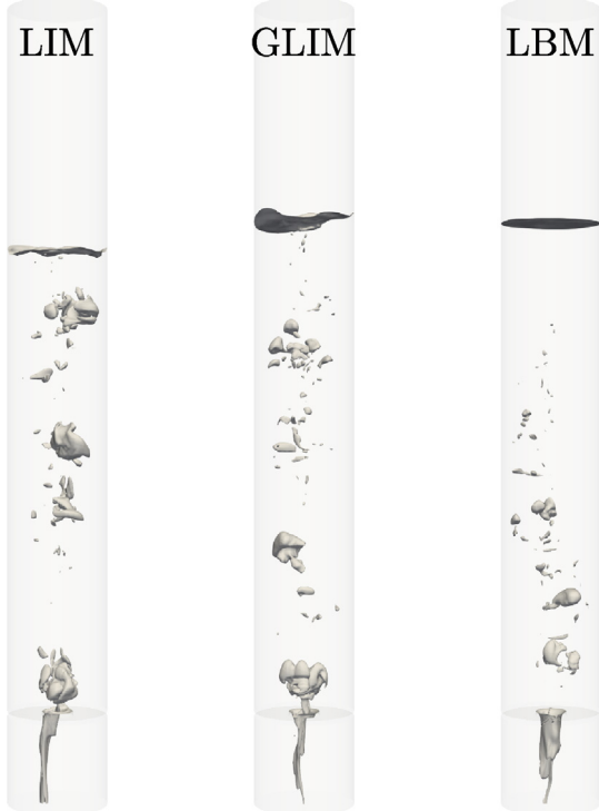
Fig. 10. Visualization of the large bubbles in the water column at t = 4.2 s. Interfaces are identified with the iso-contour \alpha_{cl} = 0.5 .
