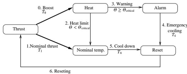
**Figure 2.** Discrete automaton representing the behaviour of a thruster sub-system. The temperature increments are uncertain in the two thrusting states and in the two cooling states.
