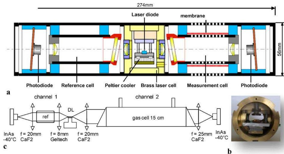
with two  $\text{CaF}_2$   $f = 20\ \text{mm}$  lenses. As the sensor was developed in the spectral range from  $2.3\ \mu\text{m}$  to  $4\ \mu\text{m}$ , InAs photodiodes were used as photodetectors. These devices are Peltier-cooled at  $-40^\circ\text{C}$  and have a detectivity ( $D^*$ ) of  $2 \times 10^{10}\ \text{cm Hz}^{1/2} \text{W}^{-1}$  at  $3\ \mu\text{m}$ . All components (Laser diode and InAs photodiodes) are temperature controlled by a PID (LDT 5910B).
