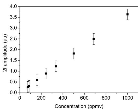
**Fig. 8**  $2f$ -WMS Calibration curve,  $\text{CH}_4$  absorption
