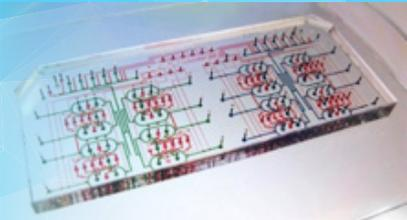
**Wu Lab-designed microfluidic device for capturing cells...**
