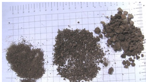
Fig. 4. Micro (<1 mm), meso (1–4 mm) and macro (>4 mm) soil aggregates. From Zanella et al. (2018d)
