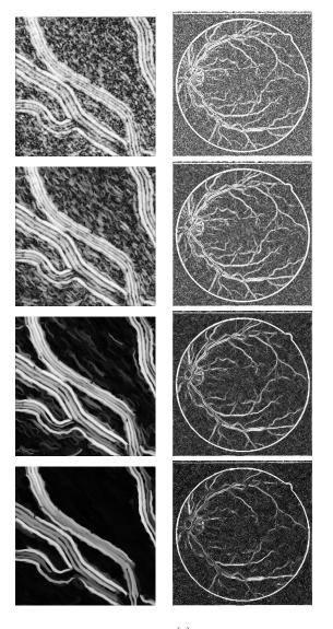
**Fig. 3**. Examples of openings  $\gamma_W^{(p)}$  on anisotropy images, in the case of a binary and symmetric matrix W, computed as explained in Section 3. For each column, from top to bottom: p=0 (original anisotropy image), p=1,5,10.
