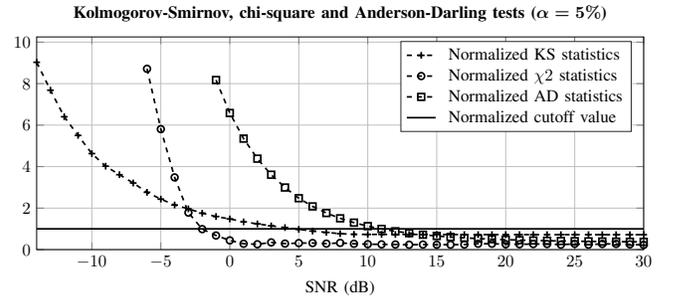
Fig. 2: Comparison of KS,  $\chi^2$  (with 2500 bins) and AD tests between the empirical distribution of  $\hat{f}_{\text{ml}}$  and the asymptotic Student-t distribution versus SNR. The cutoff value is computed for a level of significance  $\alpha = 0.05$ . All the tests are normalized by their respective cutoff for comparisons purposes.
