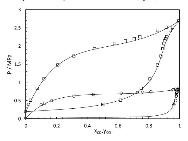
**Figure 3.** Phase diagrams (P-x-y) for N<sub>2</sub> (1) - NO (2) mixture (symbols: experimental work,  $\Box$ : data measured in this work at 127.14 K,  $\circ$ : data measured in this work at 105.69 K,  $\times$ : Data from Scheunemann and Wagner measured at 119.55K<sup>18</sup>, +: Data from Scheunemann and Wagner measured at 113.85K<sup>18</sup>, Black lines: PR-EoS with a temperature dependent BIP).
