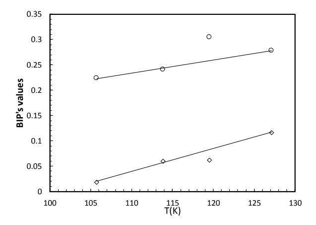
Figure 4. BIP's values with PR-WS-Wilson EoS as function of temperature. (symbols:  $\circ$ :  $\tau$ 12 ,  $\Box$ :  $\tau$ 21) for N<sub>2</sub> (1) - NO (2) mixture.
