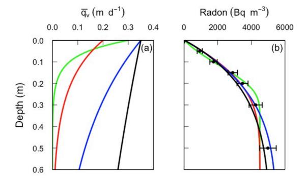
Figure 6: Simulated  $\overline{q_v}$  at different depths from 4 different radon profiles that could be accommodated within the analytical uncertainties of radon measurements of Pz1. Model parameters are q=0.35, k=0.5,  $\gamma$ =950 (Black line), q=0.35, k = 2,  $\gamma$ =1000 (Blue), q=0.2, k=0.5,  $\gamma$ =820 (Red), q=0.15, k=15,  $\gamma$ =820 (Green). All simulations use  $\theta$  = 0.4.
