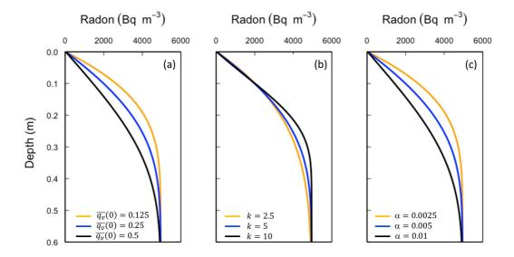
Figure 5. Sensitivity of radon profiles in Pz1 to (a) surface water – sediment exchange flux  $(\overline{q}_{\nu}(0))$ , (b) attenuation of water flux with depth (k), and (c) implicit dispersivity ( $\alpha$ ).
