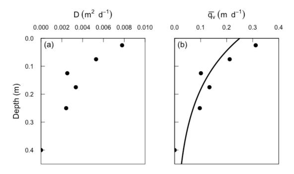
Figure 7. a) Calculated enhanced dispersion coefficient as a function of depth for Pz1 and b) comparison of the water fluxes  $(\overline{q_v})$  at different depths derived from the dispersion approach (circles) and the advective cycling model (solid line).
