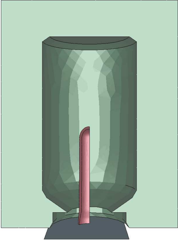
Figure 14 : Geometries of the preform and the mold.
