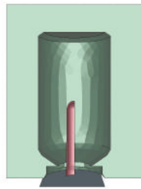
Fig. 7. Geometries of the preform and the mold.
