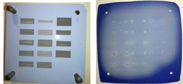
Fig. 13. Prototype stacking layer 10 with the top heat pipe grooves (left) and the full prototype after firing (right).
