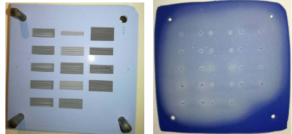
Fig. 13. Prototype stacking layer 10 with the top heat pipe grooves (left) and the full prototype after firing (right).
