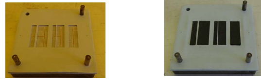
Fig. 4. Stacking of all the first 15 layers; before the insertion of the fugitive tape (left), after insertion of the fugitive tape (right).
