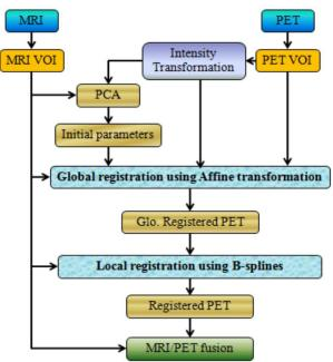
Figure 2: Flow diagram of the PET-MR registration
