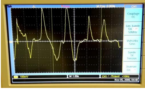
Figure 2 Photograph of the harvested random shape voltage.
