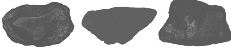
Figure 7: Three scanned ballast grains (provided by SNCF).
