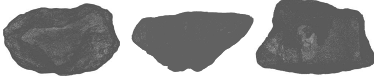
Figure 7: Three scanned ballast grains (provided by SNCF).
