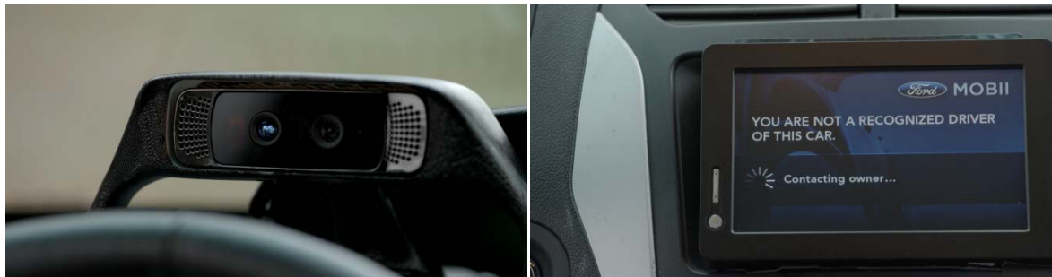
Figure 38: Facial recognition camera (left) and Mobii system informs owner that does not recognise driver (right)
