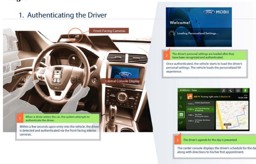
Figure 37: Driver authentication via facial recognition (Project Mobii)
