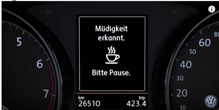
Figure 22: Visual and acoustic warning when the system finds the driver is waning (source: https://www.youtube.com/watch?v=W12qBrtypb8 )
