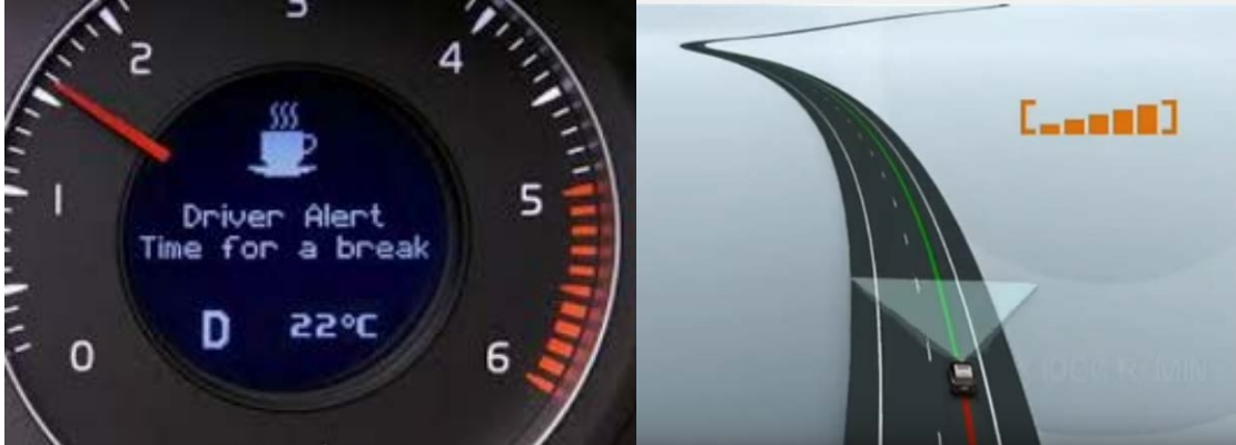
Figure 17: Volvo’s Driver Alert linked symbol (left) and camera continuously recognises lane markings (right) (Source: https://www.youtube.com/watch?v=EJA1KSrhzNU )
