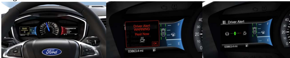
Figure 18: Ford's Driver Alert warning Technical specifications / requirements
