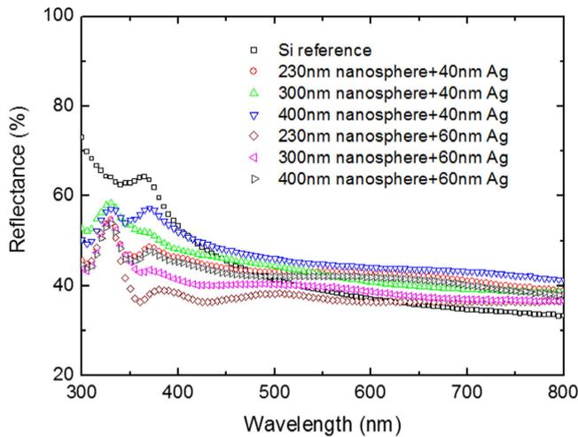
**Figure 4.** Reflectance of Ag-NP arrays for different Ag thicknesses (40 and 60 nm) and different nanosphere diameters (230, 300 and 400 nm).
