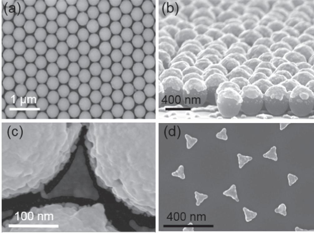
**Figure 2.** SEM images of (a) SiO<sub>2</sub> nanosphere monolayer. (b) SiO<sub>2</sub> nanospheres coated by Ag film after thermal evaporation. (c) Top-view SEM image of Ag deposition. (d) Ag-NP array after the removing of the SiO<sub>2</sub> nanospheres.
