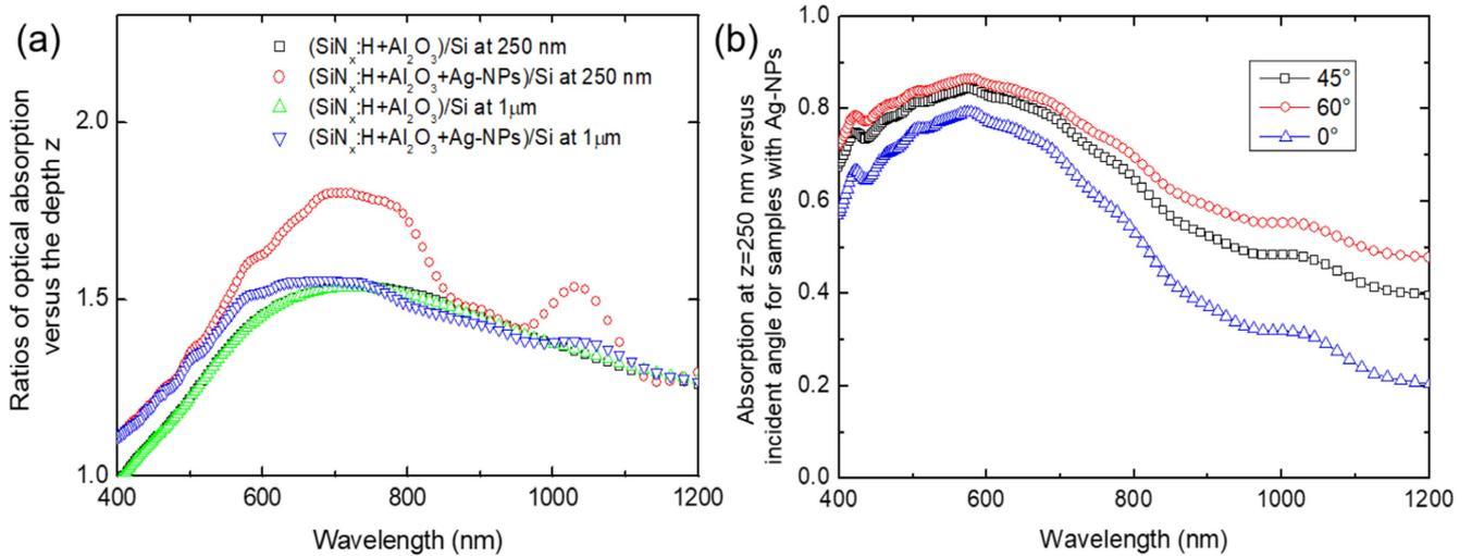
**Figure 7.** (a) FDTD simulations of the ratios of the optical absorption at depth  $z = 250$  nm and  $z = 1 \mu\text{m}$  for  $(\text{Si}+\text{Al}_2\text{O}_3/\text{SiN}_x:\text{H})$  and  $(\text{Si}+\text{Ag-NPs}+\text{Al}_2\text{O}_3/\text{SiN}_x:\text{H})$  over Si. (The Ag NPs size is 60 nm). (b) FDTD simulations of the optical absorption at  $z = 250$  nm versus the incident angle for a sample with Ag-NPs.
