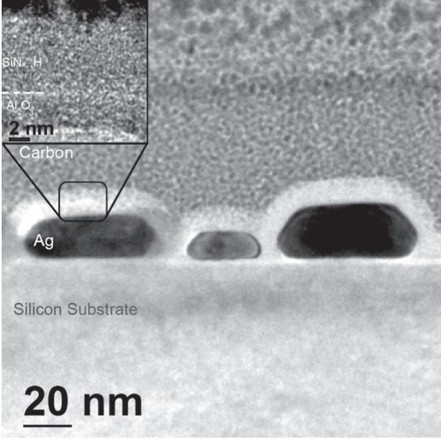
**Figure 8.** TEM image of the Si+Ag-NPs+Al<sub>2</sub>O<sub>3</sub>/SiN<sub>x</sub>:H stacks. In the inset is shown the interface between Ag-NP and Al<sub>2</sub>O<sub>3</sub>/SiN<sub>x</sub>:H layers under unfocused approach to separate both layers. The carbon layer on top of the Al<sub>2</sub>O<sub>3</sub>/SiN<sub>x</sub>:H stacks has been added for FIB preparation.
