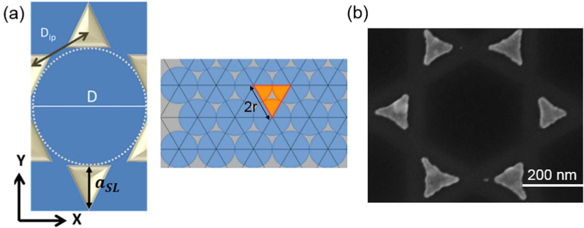
**Figure 3.** (a) Scheme for the FDTD simulation of the unit cell with the geometrical parameters of a metallic NP and an overview of the NP array. (b) SEM image of a part of Ag-NP array obtained from SiO<sub>2</sub> nanospheres with diameter  $D$  of 400 nm.
