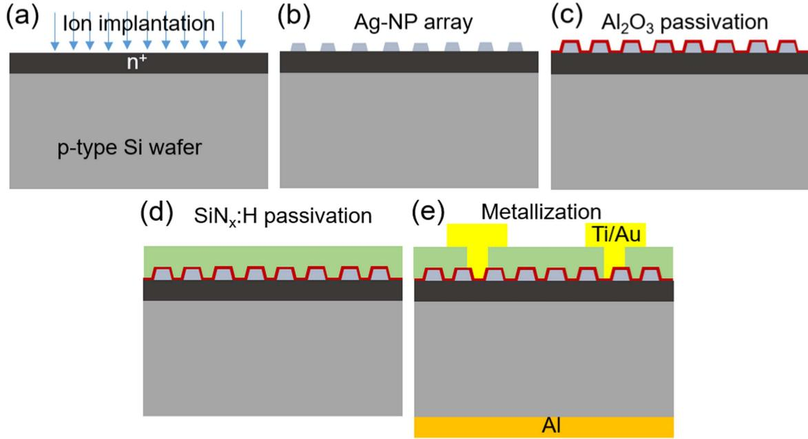
**Figure 1.** Schematic of fabrication process of Ag-NPs based implanted Si  $n^+$ -p junction. (a) Formation of  $n^+$  top layer on p-type Si wafer, (b) Ag-NP arrays deposited by NSL technique and thermal evaporation, (c) deposition of  $Al_2O_3$  tunneling layer by ALD, (d) deposition of  $SiN_x:H$  passivation layer by PECVD, (e) front and back side metallization.
