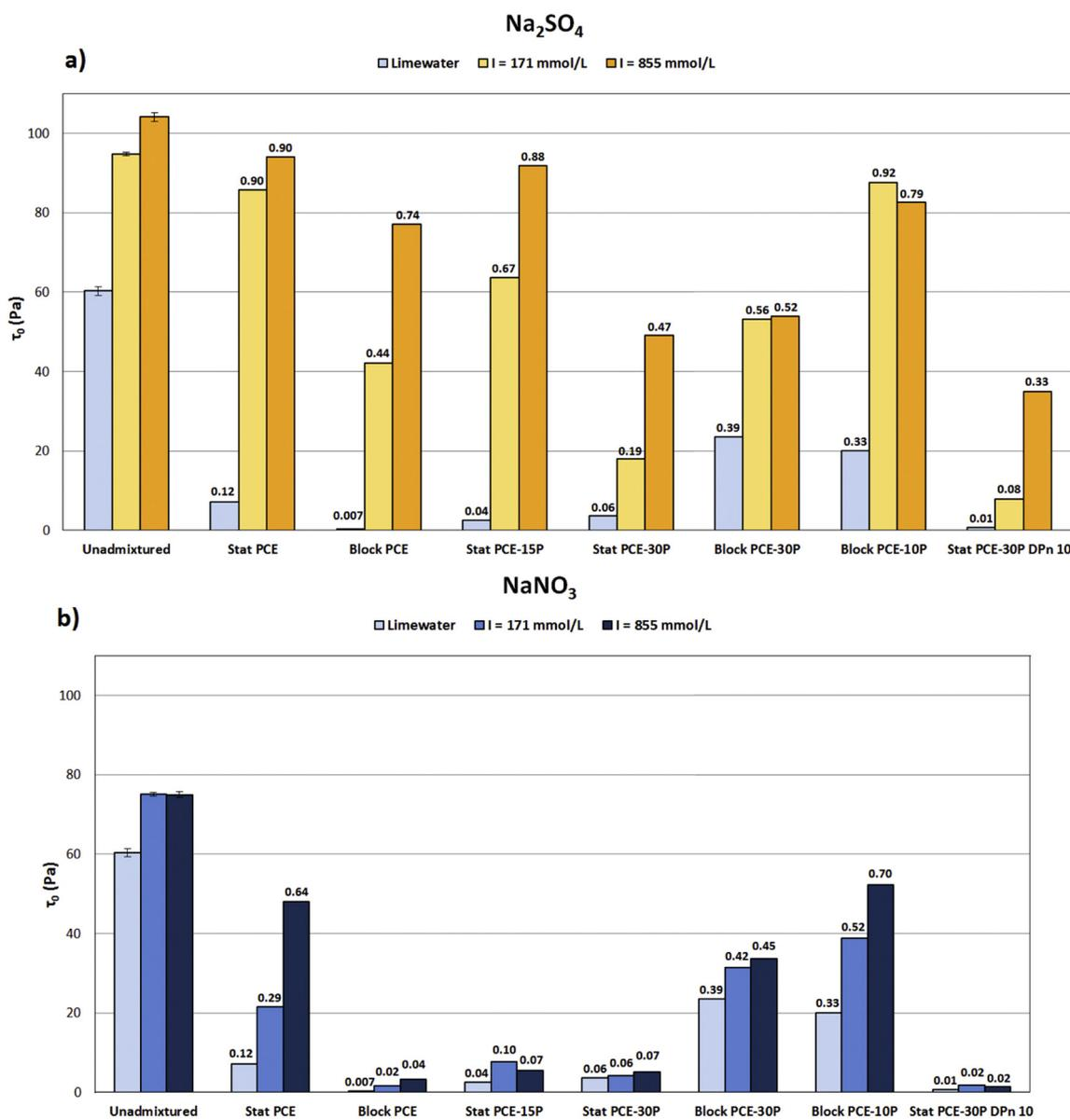
**Fig. 5.** Yield stress of calcite suspensions with 0.05% of superplasticizer for different ionic strength with sulfates (a) or with nitrates (b). The number above corresponds to yield stress of admixed suspension divided by yield stress of corresponding unadmixed suspension.
