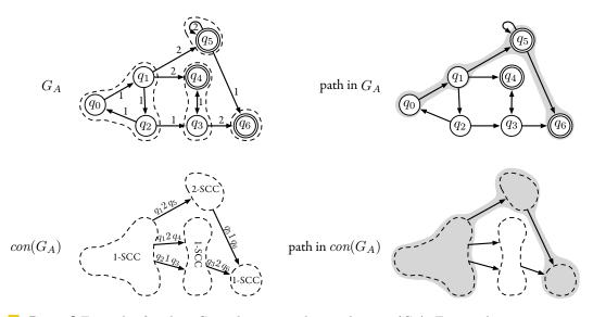
**Figure 3** Example of path in  $G_A$  and corresponding path in  $con(G_A)$ . For simplicity, we assume that the alphabet is singleton  $\mathbb{A} = \{a\}$ , and we therefore omit 'a' in the transitions.
