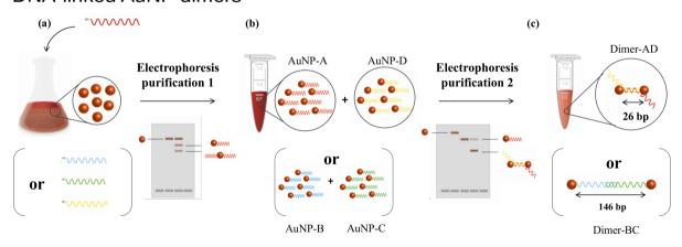
**Figure S1.** Schematic representation of the synthesis and purification of the four monomer ssDNA-AuNP monoconjugates, and the two DNA-linked AuNP dimers with interparticle links of 26 ('short link' AD) resp. 146 bp ('long link' BC).
