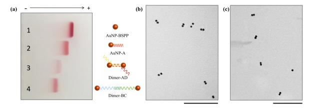
**Figure S4.** (a) Agarose gel electrophoresis (1.75% in 0.5xTBE) for the purification of DNA-AuNP dimers. With Lane 1-  $12 \pm 3$  nm BSPP AuNPs, Lane 2- Strand A ssDNA-AuNP monoconjugates (AuNP-A), Lane 3- AD DNA-AuNP dimers and Lane 4 - BC DNA-AuNP dimers. TEM images: (b) AD and (c) BC DNA-linked 12 nm AuNP dimers. Scale bars are 200 nm.
