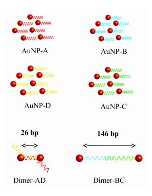
**Figure 1.** Single-stranded DNA-gold nanosphere monoconjugates (AuNP-A, AuNP-B, AuNP-C, AuNP-D), and the corresponding DNA-linked dimers with interparticle links of 26 ('short link' AD) resp. 146 bp ('long link' BC). DNA base sequences can be found in the Supporting Info.
