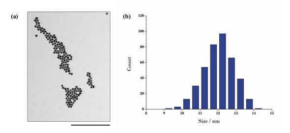
Figure S2. (a) TEM picture and (b) Size distribution histogram of  $12 \pm 3$  nm gold nanoparticles synthesised using the Turkevich method. Scale bar is 200 nm and total count is 400 particles
