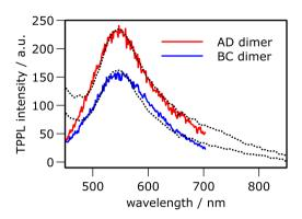
**Figure 4.** Two-photon photoluminescence spectra from DNA-linked dimers (concentration 3.5 nM in water, excitation: 800 nm, 80 MHz, 100 fs pulses). The dotted lines are the corresponding linear light scattering spectra, scaled for comparison.
