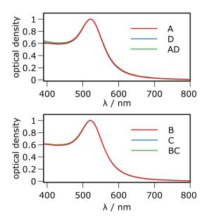
**Figure 2.** Normalized extinction spectra of ssDNA-gold nanoparticle monoconjugates and their resulting DNA-linked dimers in aqueous solution, average gold core diameter 12 nm. Top: short-link dimer AD; Bottom: long-link dimer BC. There is virtually no difference in the extinction spectra of the monomer AuNP and the dimers.
