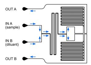
**Figure S6**. Microfluidic circuit used for the determination of diffusion coefficients. Blue arrows indicate fluid flow direction. The length of the flow interaction zone is 50 mm, with width 200  $\mu$ m and height 140  $\mu$ m. After splitting the flow, each channel follows a long serpentine channel for additional hydrodynamic resistance.
