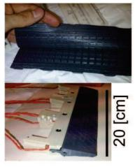
(b) HFVTE silicone cover and final HFVTE actuator
