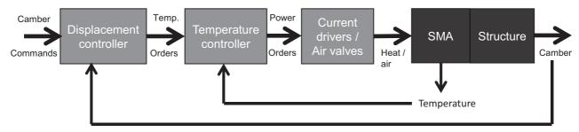
Fig. 3: Control loop architecture of camber control actuator
