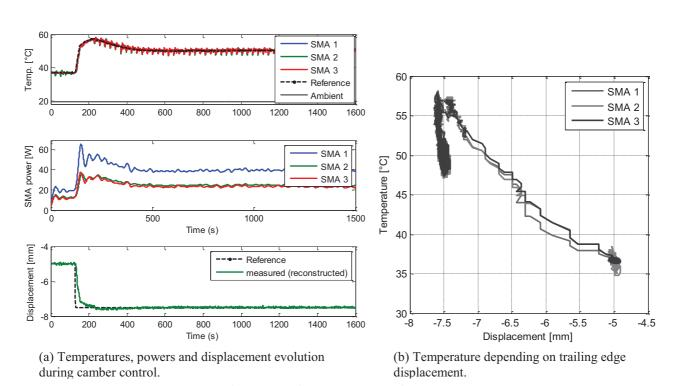
Fig. 6: Camber actuator performance
