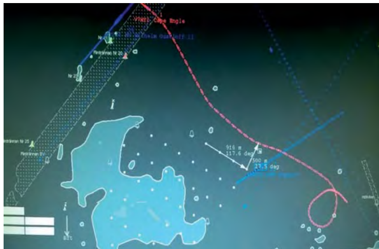
Fig. 6 – Measuring the distance between a turbine and vessel.
