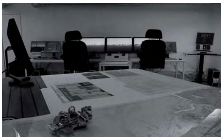
Fig. 1 – The ship handling simulator. Note the control panel between the two navigators' chairs. The three screens in the centre provide the 'outside' view as one would see from a ship realistically. On either side are 'equipment' screens showing the radar and AIS interfaces, amongst others.
