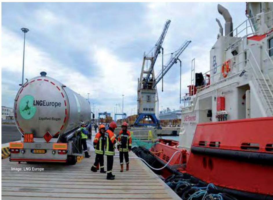
Figure 5 – Bunkering operation of an LNG powered vessel Source: LNG Europe.
