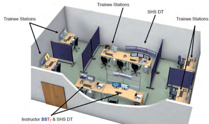
Fig. 2 – Configuration of the combined Ship-handling and Safety and Security Training Simulator
