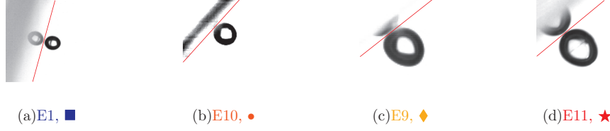
FIG. 6. Images for all bubbles in the sliding motion, at an angle just below the transition. The symbols are according to Table I. (a) E1, Re_w = 106 , We_w = 1.07 , and \theta = 75^\circ ; (b) E10, Re_w = 311 , We_w = 0.71 , and \theta = 50^\circ ; (c) E9, Re_w = 522 , We_w = 1.57 , and \theta = 40^\circ ; and (d) E11, Re_w = 627 , We_w = 1.63 , and \theta = 40^\circ . Images are shown on the same scale.
