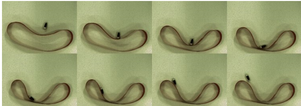
FIG. S 10. Collision of a rod with a flexible boundary. The whole duration from the upper left to the bottom right image is 1.3s. The images are separated by 0.2s except for the last two where the interval is 0.1s. The boundary is 0.1mm thick paper. Note that the rod deforms and pushes the boundary before reorienting to become parallel to it and move along the wall before escaping.
