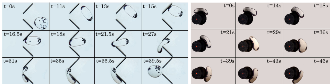
FIG. 5. Collective motion. For a flexible arena made of a boundary with 0.1 mm thick steel walls with R = 21 cm, the rods reside longer at the surface and form a cluster relatively quickly, deform the arena, and set it in motion to go through an aperture (left series) or go around an obstacle (right series). For each case, a time series is shown.
