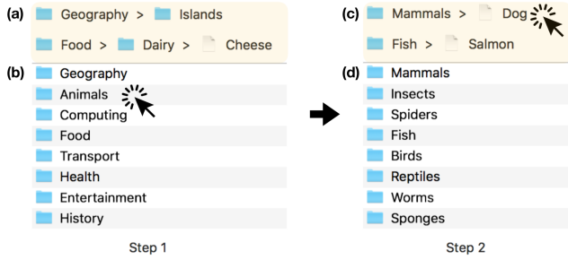
Figure 1. The BIGFile interface as the user navigates to “Dog” in a file retrieval task. (a) and (c) show the adaptive part with two shortcuts, (b) and (d) the static part. In Step 1, the shortcuts do not help and the user selects “Animals” in the static part, leading to Step 2 where the user directly selects “Dog” in the first shortcut, saving one step.
