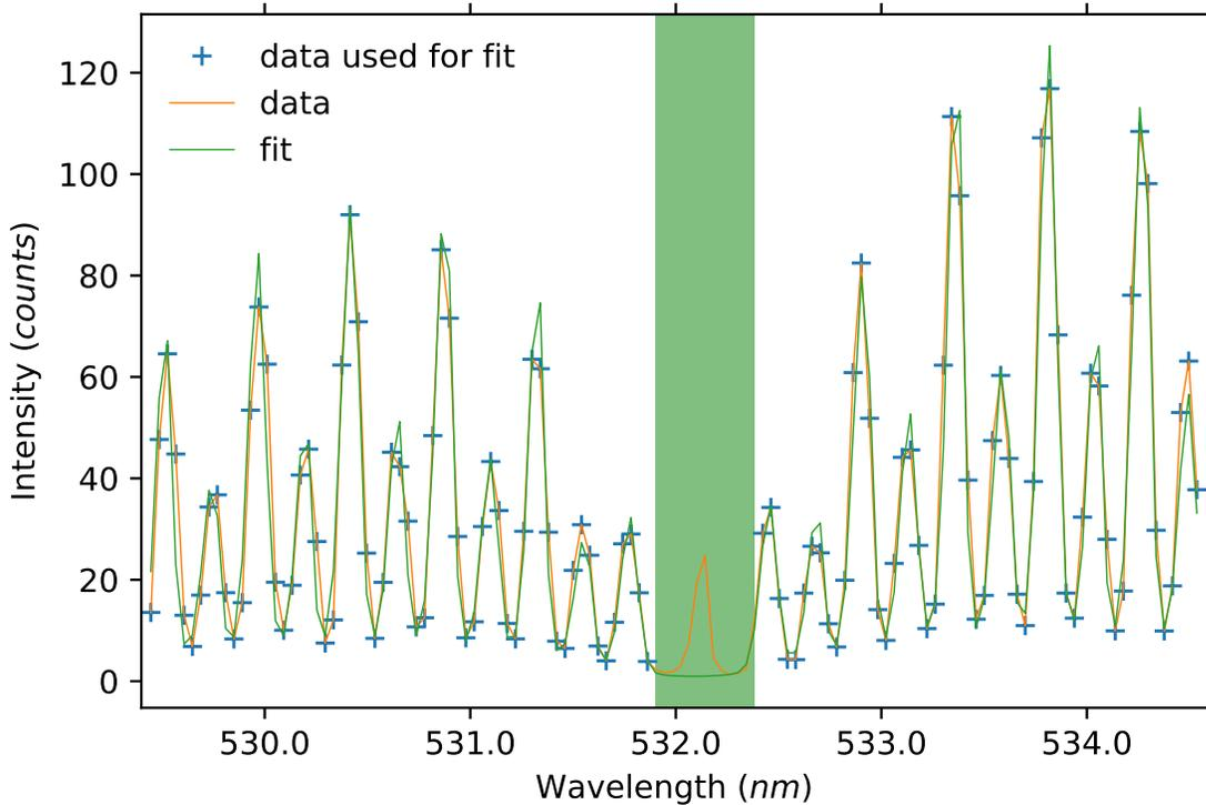
Figure 3. Raman scattering spectrum used for calibration, obtained for nitrogen at 10 mbar and a spectrometer slit width of  $300 \mu\text{m}$ . The green bar at the center of the spectrum shows the region in which points are excluded from the fit.
