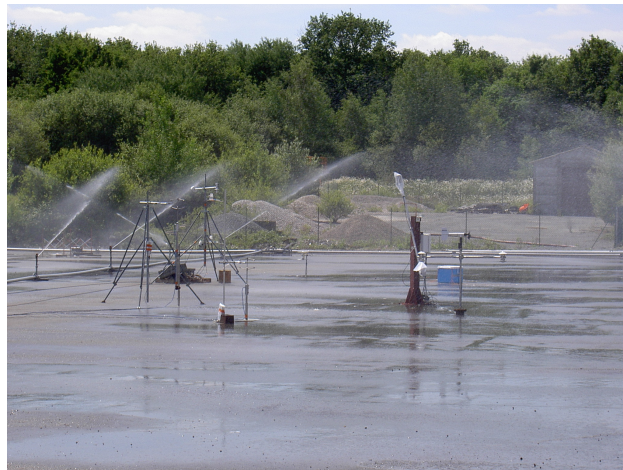
Figure 3: View of the experimental site during a watering event (an asphalt parking lot of 2500m^2 )
