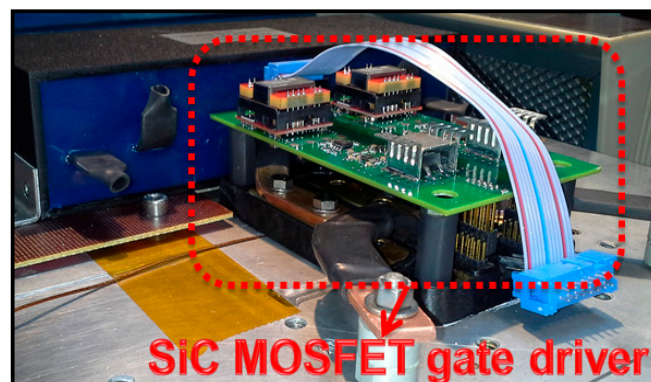
Figure 10. Gate driver of SiC module.
